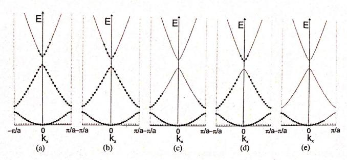
Consider the following 1D electronic band structures with filled electronic states as indicated by the closed circles. For each case, write whether the electrical current density in the x-direction  $J_x$  is zero, positive, or negative.
