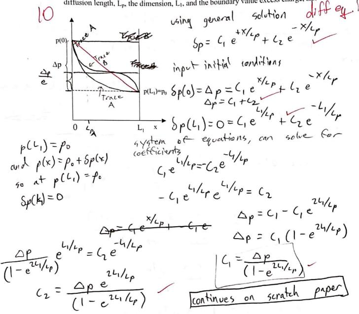
b. (10 pts) VERY IMPORTANT - Draw p(x) from 0 to L<sub>1</sub> on a <u>linear scale</u> for: two cases A) L<sub>1</sub> = 10L<sub>p</sub> (L<sub>1</sub> >> L<sub>p</sub>) AND B) L<sub>1</sub> =0.1L<sub>p</sub> (L<sub>1</sub> << L<sub>p</sub>). (Use the graph above and label the traces A and B) (Next page for part c !!!)
