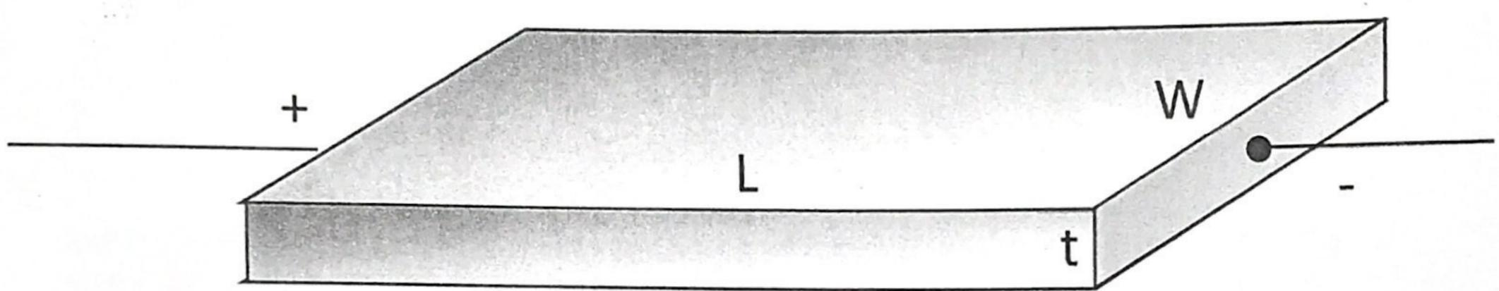
(10 pt) Consider a semiconductor resistor at 300K as shown above. If the resistor is made of intrinsic indium antimonide, InSb, and L=W=100 μm, t=0.1 μm, what is the this is true because >>MP resistance from end to end. Answers within +/- 5% get full credit.
