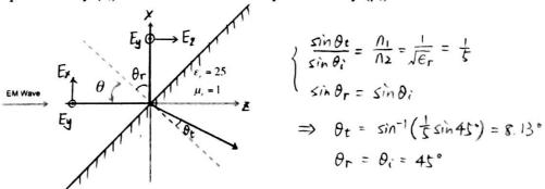
(1) [2 points] Draw two arrows representing the directions of the reflected and transmitted waves if  $\theta = 45$  degree. Please indicate the angles on the figure.
