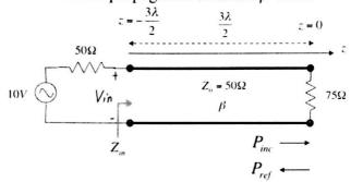
(1) [8 points] Find the voltage V(z) as a function of z, where z is from  $-3\lambda/2$  to 0.
