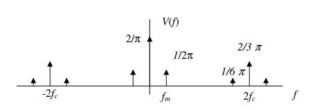
The minimum and maximum values of r(t) can then be obtained by noting that the LPF will pass only the three delta functions near the origin, leaving a time domain signal  $r(t) = \frac{2}{\pi} + \frac{1}{\pi} \cos 2\pi f_m t$ , which will have maximum  $\frac{2}{\pi} + \frac{1}{\pi}$  and minimum  $\frac{2}{\pi} - \frac{1}{\pi}$ .
