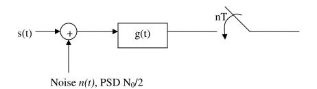
Let  $\hat{n}(t)$  be the filtered noise output. Compute the output noise power  $E[\hat{n}^2(t)]$  measured at the sampling instants nT.
