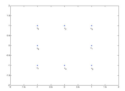
c) (10 points) The transmitted signal is corrupted by AWGN with power spectral density  $N_0/2$ , and the receiver performs maximum likelihood detection. Assume each symbol is transmitted with equal probability. Provide a signal space plot showing the locations of the symbols as well as the decision boundaries.
