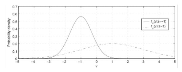
If the receiver decides that the transmitted signal was +1, this decision can either be correct or incorrect. The probabilities of being correct or incorrect depend on the values of the respective pdfs at v=-5.
