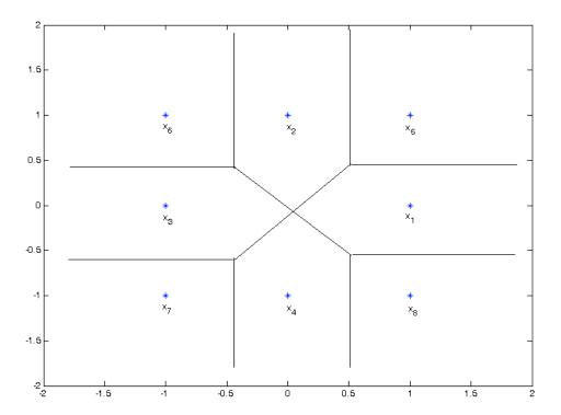
d) (8 points) Compute the tightest possible union bound on the overall probability of symbol error for this constellation assuming AWGN and that all symbols have equal probability. Your answer should be a single number (or maximally simplified expression in terms of the Q or erfc functions) that provides the average probability of symbol error, given that all symbols are equally likely to be transmitted.
