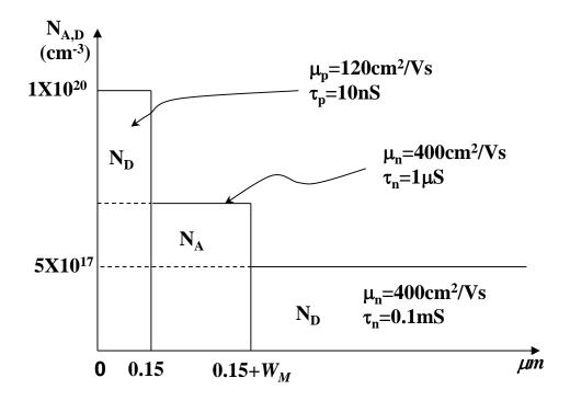
If the common emitter current gain,  $\beta_o$ , measured with V<sub>BE</sub>=0.7V and V<sub>BC</sub>=0V, is 80, and the Early voltage is 50V, what are  $N_A$  and W<sub>M</sub>? (25 points)
