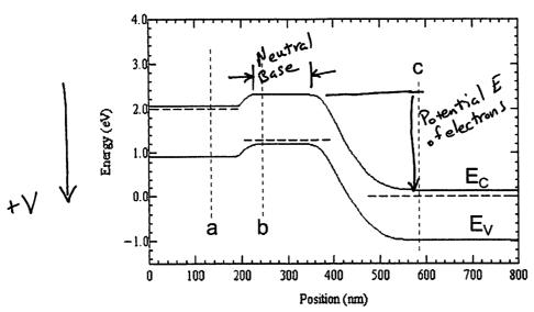
The plot above is a faithful band diagram of an electron device calculated using an accurate Poisson solver. The electron energy scale and position in the device are accurately depicted as are the conduction and valence bands and the quasi-Fermi levels (dotted lines). Use this graph to answer the questions below by inspection (no calculations are necessary). The dotted lines a, b and c are reference planes referred to below.
