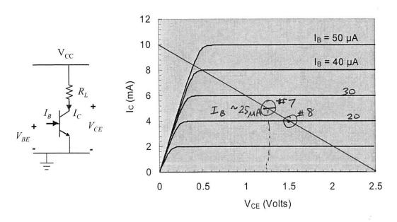
7. (4 pts.) Referring to the common-emitter Ic-Vce characteristic above. The transistor with the above characteristic is biased from (2.5V) supply (Vcc = 2.5V) with a 250  $\Omega$  load. V<sub>BE</sub> is chosen such that the base current is 25  $\mu$ A. What is the approximate collector-emitter voltage (V<sub>CE</sub>) across the transistor?
