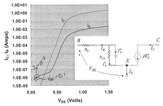
9. (4 pts.) In the transistor with measured Gummel characteristic as shown above, find the approximate base shunt resistance R<sub>EX</sub> in the model?
