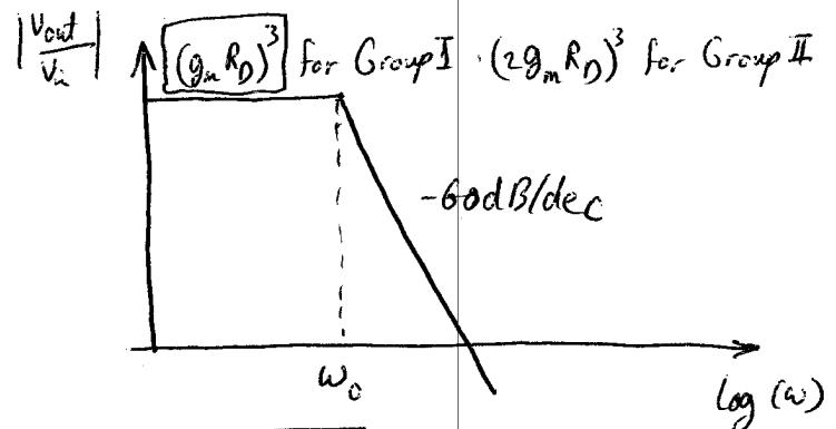
$$\left| \frac{V_{out}}{V_i} \right|(\omega_{3dB}) = \frac{1}{\sqrt{2}} \left| \frac{V_{out}}{V_i} \right|(0)$$
