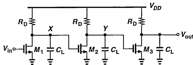
$$\frac{V_{out}(s)}{V_y(s)} = \frac{V_y(s)}{V_x(s)} = \frac{V_x(s)}{V_i(s)} = \frac{-g_m R_D}{1 + s R_D C_L} = \frac{-g_m R_D}{1 + \frac{s}{\omega_0}} \quad \text{with } \omega_0 = \frac{1}{R_D C_L}$$
