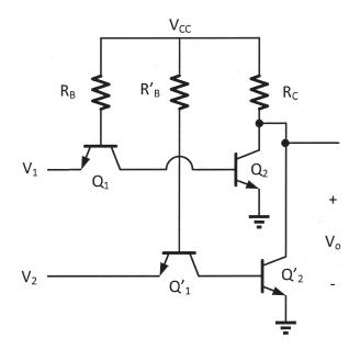
4. Calculate the bias currents, voltages, and the voltage gain of the self-biased amplifier below.  $V_{BE,ON} = 0.6V$ ,  $R_B = 10R_C = 12k\Omega$ ,  $V_{CC} = 3V$ ,  $V_A = \infty$ , and  $\beta = 9$ .
