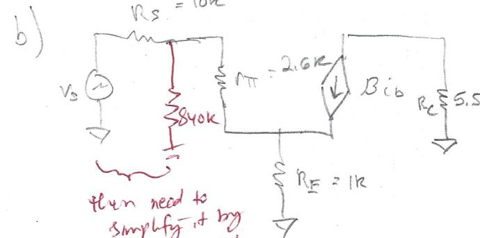
$$V_S = (R_S + r_{\pi}) i_O + R_E i_O$$
