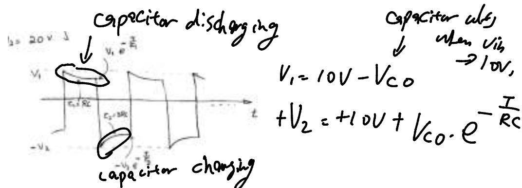
$$C_1 = RC = \frac{T}{2}, \quad C_2 = 3RC = \frac{3T}{2}$$
