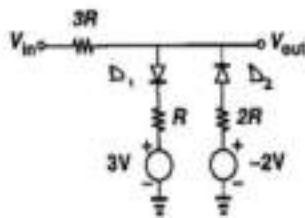
①  $V_{\text{in}} = -5 \text{ V}$ , assume  $D_1$  off  $D_2$  on
