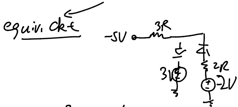
$$V_{\text{out}} = \frac{2}{5}V_{\text{in}} - \frac{6}{5}\text{V}$$
