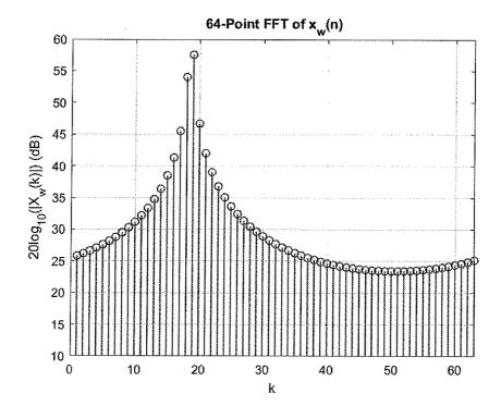
The associated continuous-time input signal,  $x_a(t)$ , could be one or more of the following signals. Identify which one(s) of the signals below could have produced this FFT. And clearly explain your reasoning for your choice(s).
