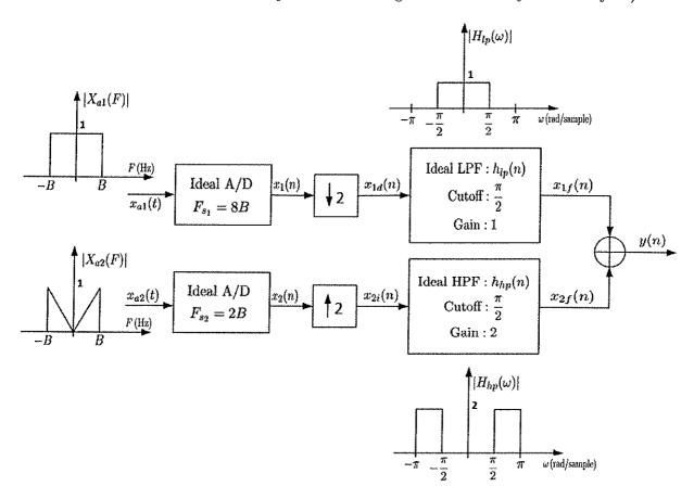
(a) (6 points) Plot the magnitude DTFT of  $x_1(n)$  and  $x_2(n)$  over  $-2\pi < \omega < 2\pi$ , showing as much detail as possible. Show the important points on the frequency axis both in terms of rad/sample as well as Hertz.
