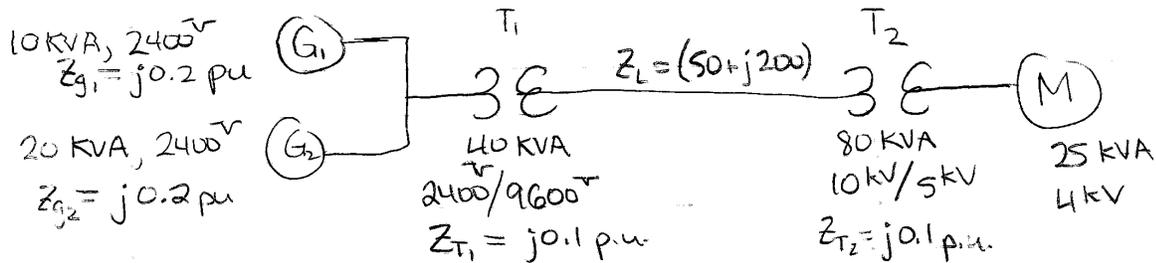
$$S_B = 100 \text{ kVA}, V_{B(G)} = 2400 \text{ V} \text{ (at generator-side)}$$
