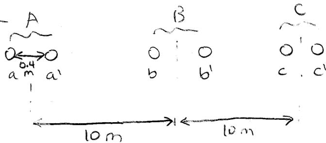
$$d = 1.108'' \quad \text{GMR} = 0.0375 \text{ ft.} \quad (D_s)$$
