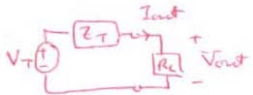
Power delivered =  $P = \frac{1}{2} \operatorname{Re}(V_{out} * I_{out}^*)$
