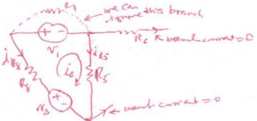
$$\text{Loop current } i_A = \frac{V_8 - V_1}{R_5 + R_8} = -i_{R_8} = i_{R_5}$$
