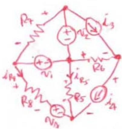
Easy ones:  $i_{R7} = \frac{1}{R7}(V_2 - V_1)$ ;  $V_{R6} = R6(i_4 - i_3)$
