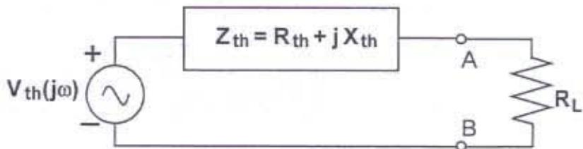
a.) Derive a formula for the required value of  $R_L$  as a function of the  $R_{th}$  and  $X_{th}$  components of the Thevenin impedance  $Z_{th}$ .
