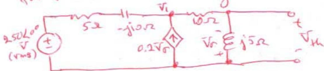
$$\left\{ \begin{array}{l} \frac{V_1 - 250}{5 - j10} - 0.2 V_o + \frac{V_1}{10 + j5} = 0 \\ V_o = \frac{-j5}{10 + j5} V_1 = \frac{-jV_1}{2 + j1} \\ -0.2 V_o = \frac{j0.2 V_1}{2 + j1} \end{array} \right. \Rightarrow V_1 [ \frac{1}{5 - j10} + \frac{j0.2}{2 + j1} + \frac{1}{10 + j5} ] = \frac{250}{5 - j10}$$
