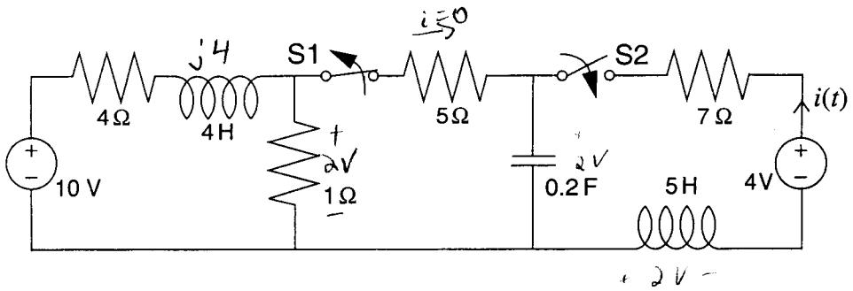
$$a) \omega_0 = \frac{1}{\sqrt{LC}} = \frac{1}{\sqrt{5H \cdot 0.2F}} = 1 \quad \omega_0^2 = 1 \quad \omega_0^2 > \omega^2 \text{ means} \\ \omega = \frac{R}{2L} = \frac{2\Omega}{2 \cdot 5H} = 0.7 \frac{\text{rad}}{\text{s}} \quad \omega^2 = 0.49 \quad \text{it is underdamped.}$$
