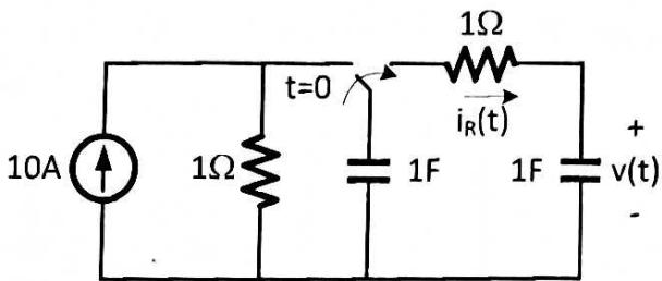
$$\begin{aligned} \text{Node Voltage: solve } E_2 \\ \left\{ \begin{aligned} 2E_1 - 10 + \frac{E_1 - E_2}{1} &= 0 \\ 2E_2 + \frac{E_2 - E_1}{1} &= 0 \end{aligned} \right. \end{aligned}$$
