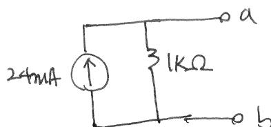
(b) Find the Thevenin equivalent of the simple transformer circuit below.
