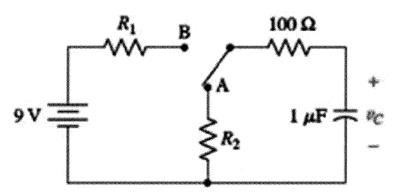
$$V_{c(0-)} = V_{c(0+)} = 0$$
