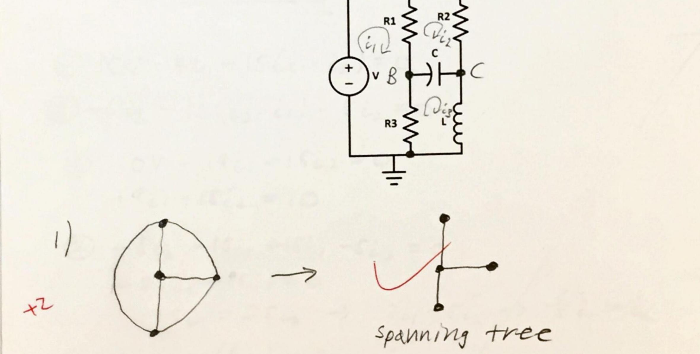
2) 4 hodes/ x2 3 chords 3 minimum node voltage centon 3) h = 4 h - 1 = 3 $V_A = V$  $\frac{+4}{R_1} \frac{V_B - V_A}{R_1} + C \frac{d(V_B - V_C)}{dt} + \frac{V_B}{R_3} = 0$  $C \frac{d(V_c - V_B)}{dt} + \frac{V_c - V_A}{R_2} + \frac{1}{L}SV_c dt = 0$
