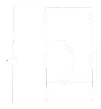
Since the circuit cannot be drown on a sheet of paper without coossing lines. it is nonplanar
