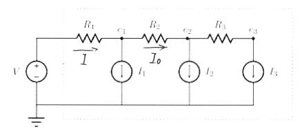
(a) Using the node method, develop a set of simultaneous equations for the power distribution network that can be solved for the three unknown node voltages e1, e2 and e3. Express these equations in the form (5 points)
