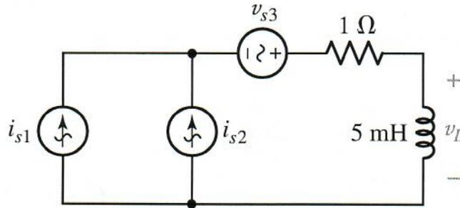
$$V_L(t) = L \frac{d}{dt} (i_{s1} + i_{s2}) = 5 \text{ mH} [-400 \sin(200t) - 100 \sin(100t)]$$
