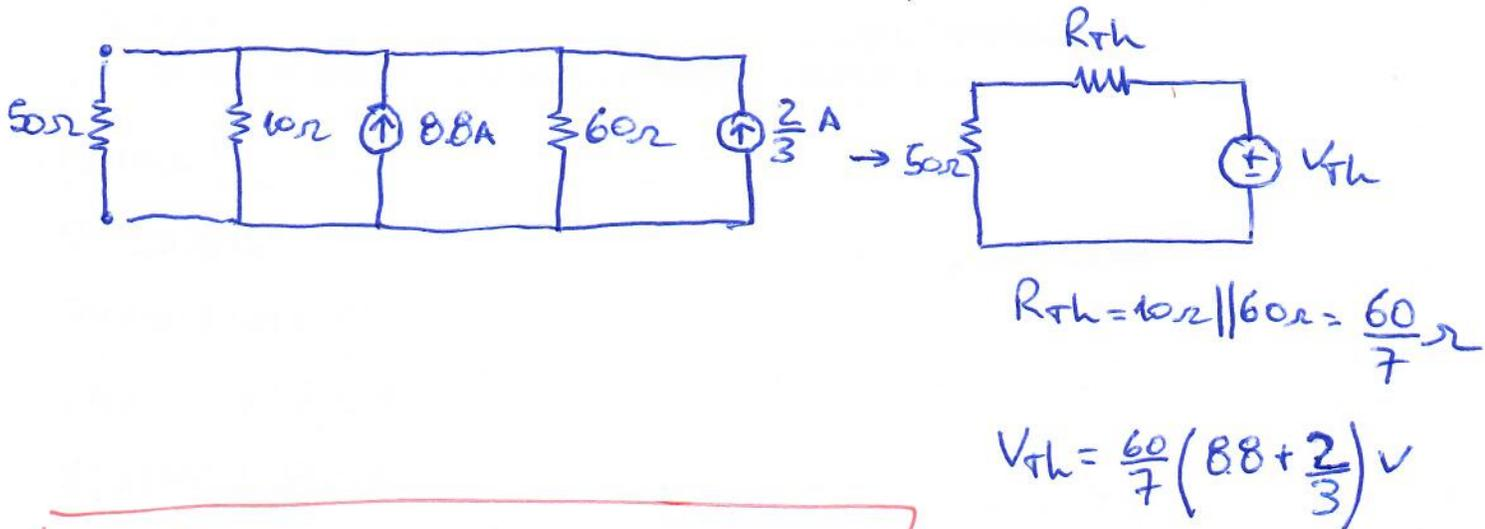
$$P_{50\Omega} = \left( V_{th} \frac{50\Omega}{50\Omega + R_{th}} \right)^2 \frac{1}{50\Omega} \approx 95.96 W$$
