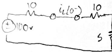
$$i_L(0^-) = \frac{100\text{V}}{25\Omega} = 4\text{A}$$
