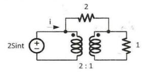
Find the current i in the circuit below by a) node analysis, b) superposition (40 points).
