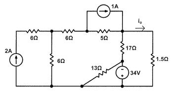
Remove 61 and 131 resistors first then apply a source transformation to each current source yields
