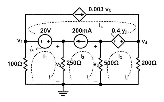
a) Make equations to find  $v_1$ ,  $v_2$ ,  $v_3$  and  $v_4$  using the node-voltage method. Use the reference node and the notation in the circuit. (7 pts)
