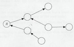
A directed tree can be represented by a reduced node-arc incidence matrix defined as follows. We label one node as the root node. The other nodes are labeled with integers from 1 to n. The arcs are also given integer labels from 1 to n. The node-arc incidence matrix A is then defined as the  $n \times n$  matrix with coefficients
