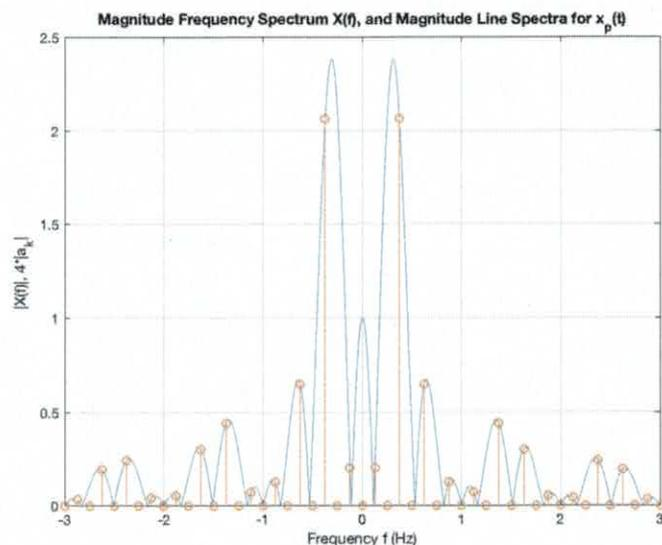
6. (18 points) Consider a complex-valued signal  $x(t) = x_I(t) + jx_Q(t)$  with its frequency spectrum  $X(f) = \mathcal{F}\{x(t)\}$  shown below:
