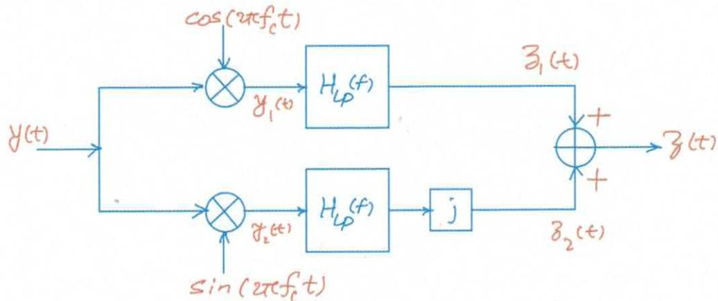
where  $H_{LP}(t)$  is the same ideal Low-Pass Filter with cut-off at  $B$  Hz as shown in Part (c). Obtain and plot  $Z(f) = \mathcal{F}\{z(t)\}$ , and prove that  $z(t)$  will indeed be equal to  $x(t)$ . This is called an *I/Q Demodulator*.
