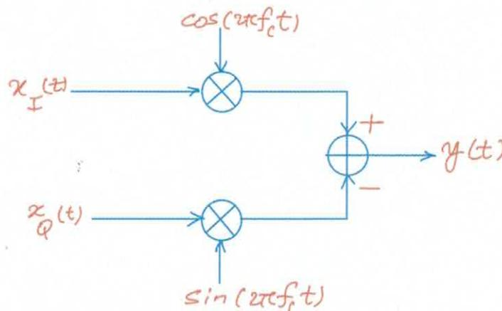
Obtain the CTFT of  $y(t)$ , i.e.,  $Y(f)$ , in terms of  $X(f)$  and plot  $|Y(f)|$ . This is called an In-phase/Quadrature or *I/Q Modulator* (Hint: Notice that  $y(t) = \Re\{x(t)e^{j2\pi f_c t}\}$  and for any complex number  $a$ , we have  $\Re\{a\} = \frac{a+a^*}{2}$ ).
