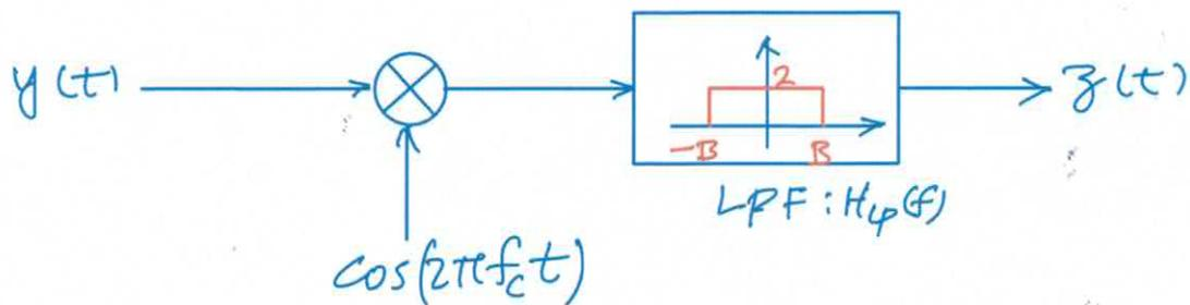
Multiplying by  $\cos(2\pi f_c t)$  shifts the spectrum back and forth by  $f_c$ . But, as shown, in this scenario, the signal will corrupt itself, and so we cannot recover our original signal  $x(t)$ .
