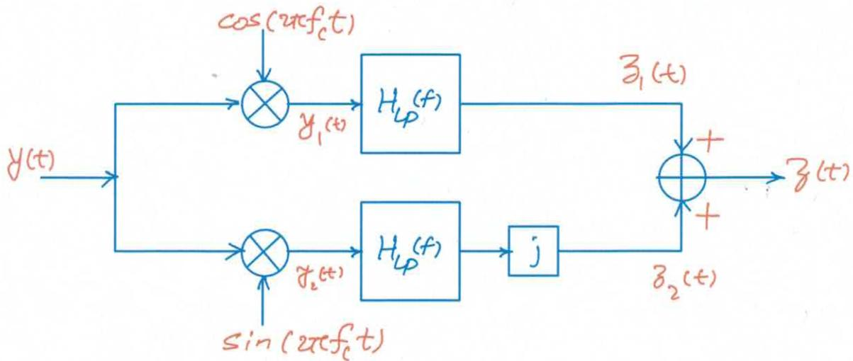
where  $H_{LP}(f)$  is the same ideal lowpass filter with cutoff at  $B$  Hz as shown in part c.
