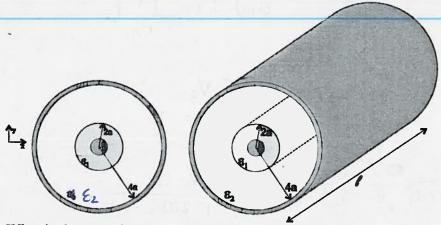
(a) (20 points) What is the capacitance C between the inner and outer conductors? (Your answer should be in terms of only geometric and material parameters such as  $\angle a, \varepsilon_1, \varepsilon_2$ )
