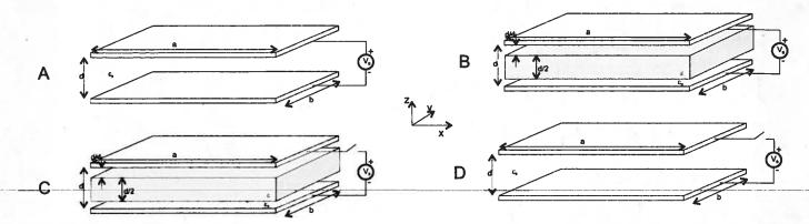
(a) (10 points) Consider the following parallel plate capacitor with perfectly conducting metal plates, and only vacuum in between as shown below in figure (A). Assume the plates are held at a constant potential difference  $V_0$  using a voltage source. Give an expression for the electric field in the gap between the plates (don't forget vector direction) in terms of  $V_0$ , and the dimensional and material quantities (i.e.  $a, b, d, \varepsilon$ , - (NOT C!)).
