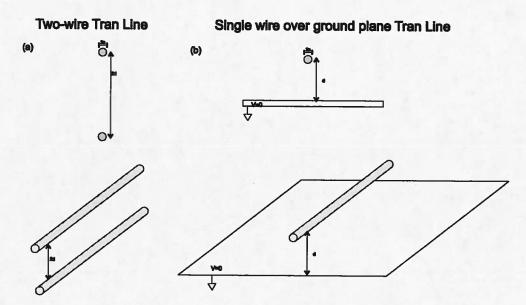
The Single wife TL is the image theory equivalent to the two wire line. However the voltage dropis 2 of the two wire case for the same charge so C=Q = 2 Cm.
