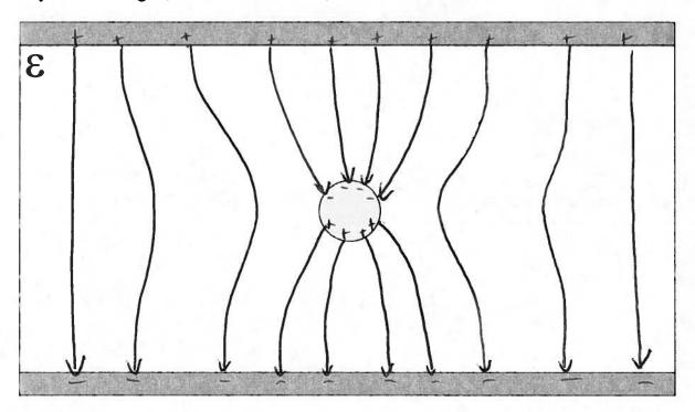
(d) (3 points) Imagine we modify a conventional capacitor by filling the dielectric with very tiny metal spheres. However, they don't touch each other, so the material remains insulating. Will the inclusion of these spheres increase or decrease the capacitance C, or will it remain unchanged? Explain why.
