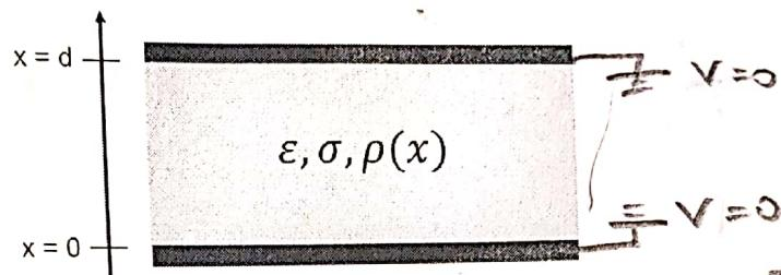
$$\textcircled{a} \quad \nabla^2 V = -\rho_0/\epsilon \rightarrow \frac{\partial^2 V}{\partial x^2} + \frac{\partial^2 V}{\partial y^2} + \frac{\partial^2 V}{\partial z^2} = -\rho_0/\epsilon$$
