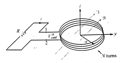
An inductor is formed by winding N turns of a thin conducting wire into a circular loop of radius a. The inductor loop is in the x-y plane with its center at the origin, and connected to a resistor R, as shown in the figure above. In the presence of a magnetic field  $\vec{B} = B_0(\hat{y}3 + \hat{z})\sin\omega t$ , where  $\omega$  is the angular frequency. Note:  $\frac{d\sin x}{dx} = \cos x$ ;  $\frac{d\cos x}{dx} = -\sin x$ Find the following parameters:
