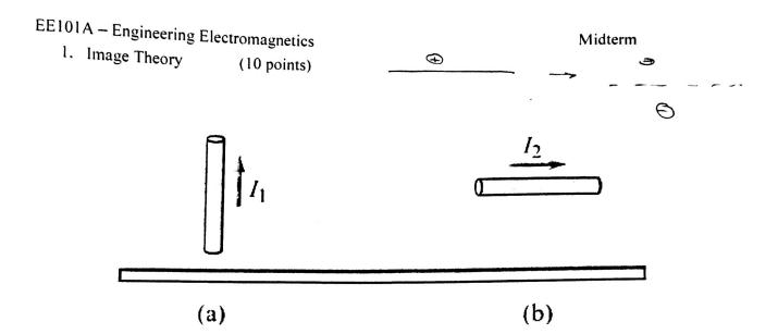
Conducting wires above a conducting plane carry currents  $I_1$  and  $I_2$  in the directions shown in the figure above. Keeping in mind that the direction of a current is defined in terms of the movement of positive charges, what are the directions of the image currents corresponding to  $I_1$  and  $I_2$ ?
