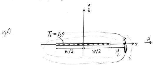
An infinitely long thin conducting sheet of width w positioned along the x direction and lying in the x-y plane as shown in the figure. It carries a surface current density of  $\vec{J}_s = J_0 \hat{y}$ . Find the magnetic field  $\vec{H}$  at point P.
