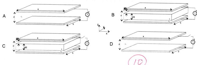
(a) (10 points) Consider the following parallel plate capacitor with perfectly conducting metal plates, and only vacuum in between as shown below in figure (A). Assume the plates are held at a constant potential difference  $V_0$  using a voltage source. Give an expression for the electric field in the gap between the plates (don't forget vector direction) in terms of  $V_0$ , and the dimensional and material quantities (i.e.  $a, b, d, \varepsilon$ , - (NOT C!)).
