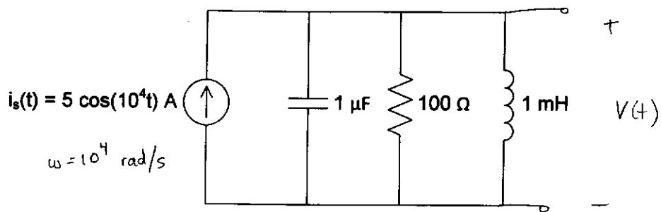
$$\begin{aligned} Z &= \frac{1}{\frac{1}{R} + \frac{1}{j\omega L} + j\omega C} = \frac{1}{\frac{1}{R} + j(\omega C - \frac{1}{\omega L})} \\ &= \frac{1}{0.01 + j(0.01 - 0.1)} = \frac{1}{0.01 - 0.09j} \\ &= \frac{1}{0.09055} \angle -83.66^\circ = 11.04 \angle 83.66^\circ \end{aligned}$$
