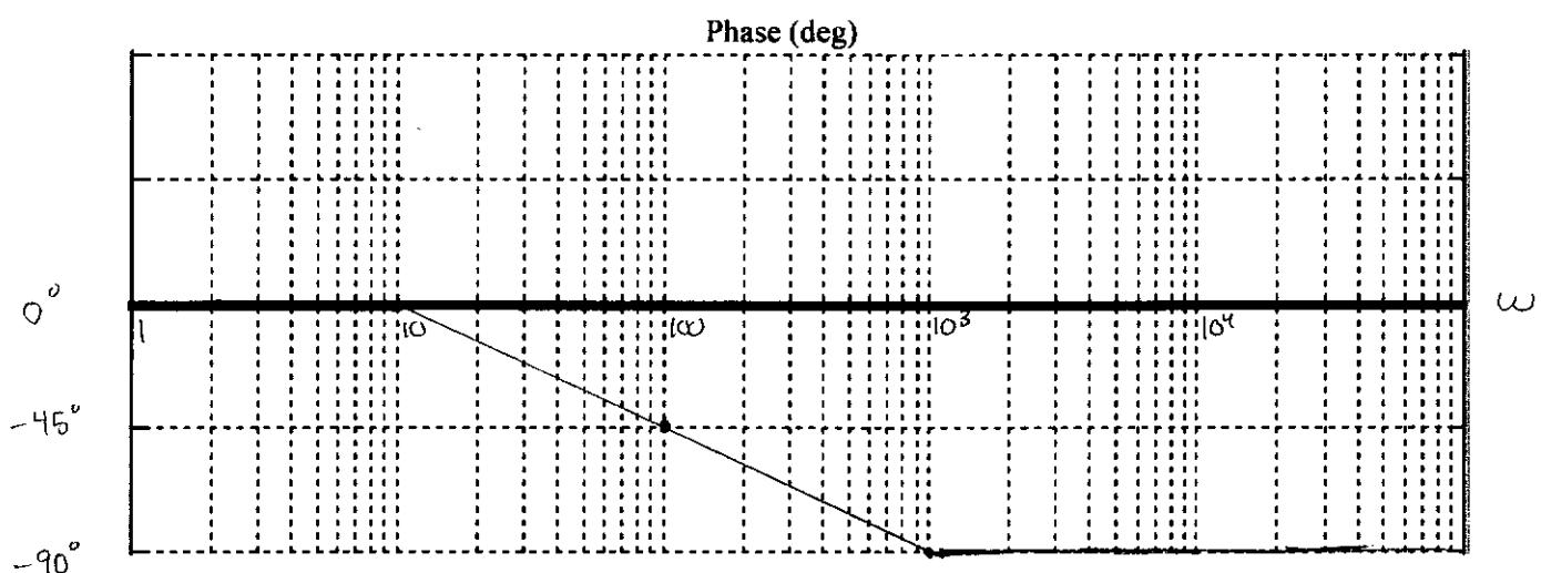
3c) Plot the magnitude and phase using Bode plots of  $H_2(\omega) = I_C/I_{IN}(\omega)$ .
