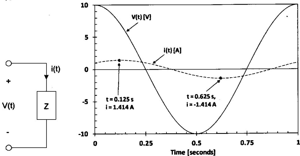
From the information given, reduce the load  $Z$  into its simplest possible configuration involving passive elements (i.e. resistors, inductors, capacitors).
