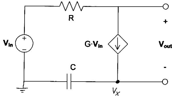
$$\underline{\text{KCL}}: \quad G\tilde{V}_{in} = \frac{\tilde{V}_x}{j\omega C} = j\omega C \tilde{V}_x$$
