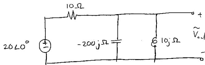
$$\begin{aligned}\tilde{V}_{out} &= 20 \cdot \frac{-200j \parallel 10j}{10 + (-200j \parallel 10j)} \\ &= 20 \cdot \frac{10.53j}{10 + 10.53j} \\ &= \frac{210.53 \angle 90^\circ}{14.52 \angle 46.48^\circ} \\ \boxed{\tilde{V}_T &= 14.5 \angle 43.52^\circ \text{ [V]}}\end{aligned}$$
