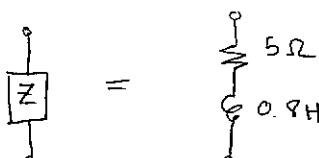
2a) Find the average power, reactive power, and apparent power delivered by the current source in the circuit below.
