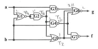
Part (a) Assuming that negated variables are available and that NAND and NOR gates have the same delays, identify the *critical path* of the network by listing its gates along the path, starting at the inputs:
