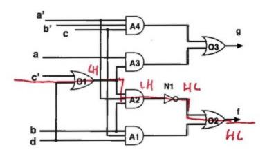
Part (a) Assuming that negated variables are available and that all gates have the same delays, identify the *critical path* of the network by listing its gates along the path, starting at the inputs:
