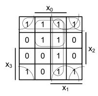
The equivalent product terms are  $x_3'x_2'$  (c),  $x_3'x_0$  (e),  $x_2'x_1$  (missing),  $x_2'x_0'$  (missing) and  $x_1x_0$  (h).
