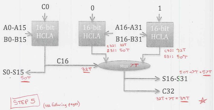
In this diagram, A0-A15 indicates the lower 16 bits of one of the input operands (A), and A16-A31 indicates the upper 16 bits of the same input operand. Note that the upper 16 bits of the two input operands are both used as input to the two 16-bit HCLAs in the right portion of the figure. S0-S31 are the sum bits, and C32 is the carry out of the 32-bit adder. Note that the output of the HCLAs is actually 17 bits – as labeled it branches off to 16 sum bits and 1 carry out bit.
