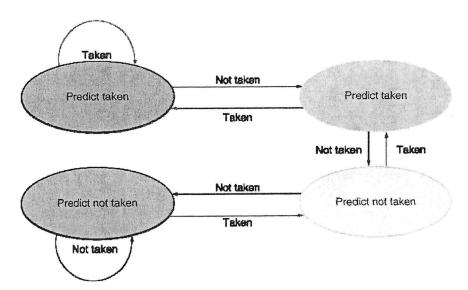
The branch predictor is accessed in the instruction fetch stage to determine whether a particular branch is taken or not taken. Assume that we have some other structure to predict whether an instruction is a branch in the instruction fetch stage, and to what target address the branch may go.
