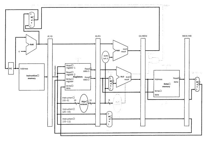
Branches are resolved in the MEM stage as shown in the figure above. Assume that instruction and data memory are perfect -i.e. accesses only take a single cycle. Further assume that the pipeline is extended to be able to handle *addi* and *j* instructions. These extensions still result in a 5-stage pipeline.
