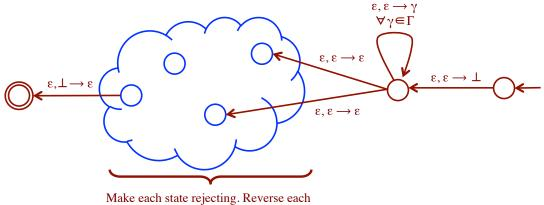
Make each state rejecting. Reverse each arrow and change its label from  $\sigma, \gamma \rightarrow \gamma'$  to  $\sigma, \gamma' \rightarrow \gamma$
