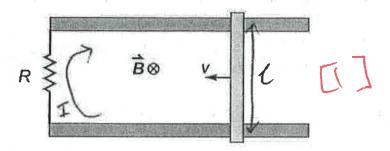
Calculate the induced current through the resistor, and indicate its direction on the figure above. [Ignore the resistance of the bar and the rails].
