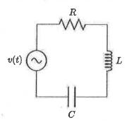
(a) Using a phasor diagram, or otherwise, obtain an expression for I, the amplitude of the current through the circuit in terms of L, R, C,  $\omega$  and V.
