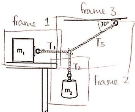
$$\frac{T_1}{\cos 30^\circ} = \frac{T_2}{\sin 30^\circ}$$
