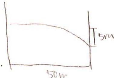
$$\begin{array}{ll} \Delta x = 50 & \Delta y = -5 \\ v_0 = 35\sqrt{2} & v_0 = 0 \\ v = 35\sqrt{2} & v = -7\sqrt{2} \\ a = 0 & a = -9.8 \\ \Delta t & \frac{5\sqrt{2}}{7} s \end{array}$$
